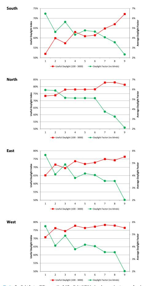
Fig 4 Daylight factor (DF) versus Useful Daylight (UDI) in 6 m deep perimeter zone for nine façade options
