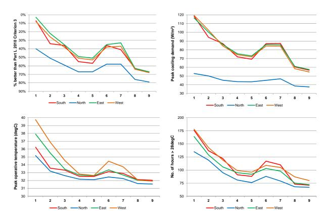
Fig 3 Thermal comfort indicators for different façade options and orientations
