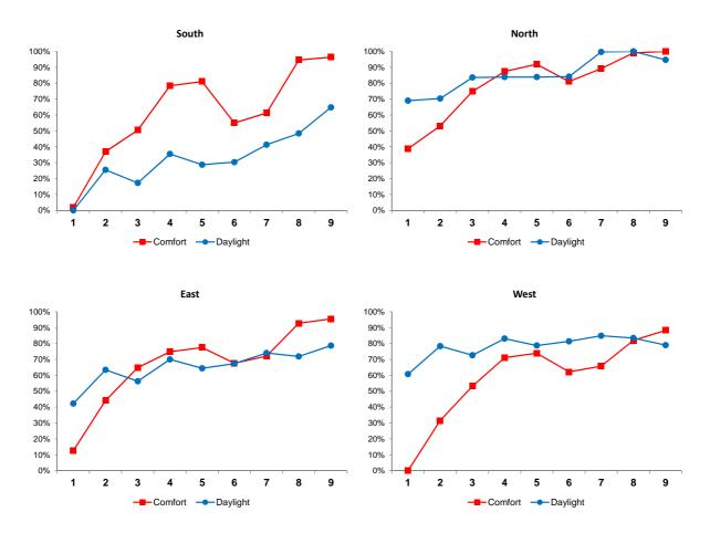
Fig 5 Thermal comfort and daylight comparative scores for nine façade options
