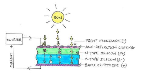
Fig 1 How a solar cell works
