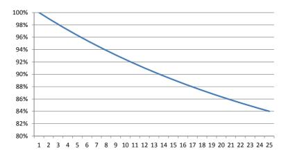
Fig 2 PV panel output degradation over time
