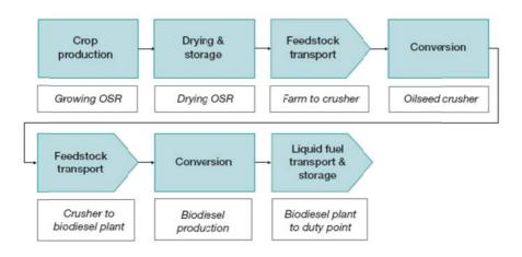
Fig 4 Example fuel chain for oil seed rape (source: UK RFA)
