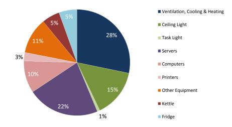
Fig C.1 Energy consumption breakdown for the 'lowest energy office'
