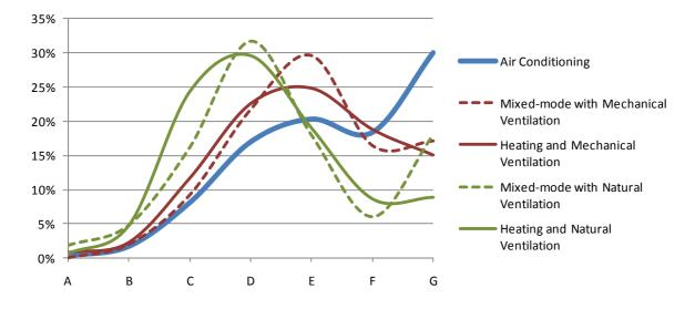
Fig C.3 Distribution of ratings by HVAC type for 2,311 'offices' from the 2010 DEC database
