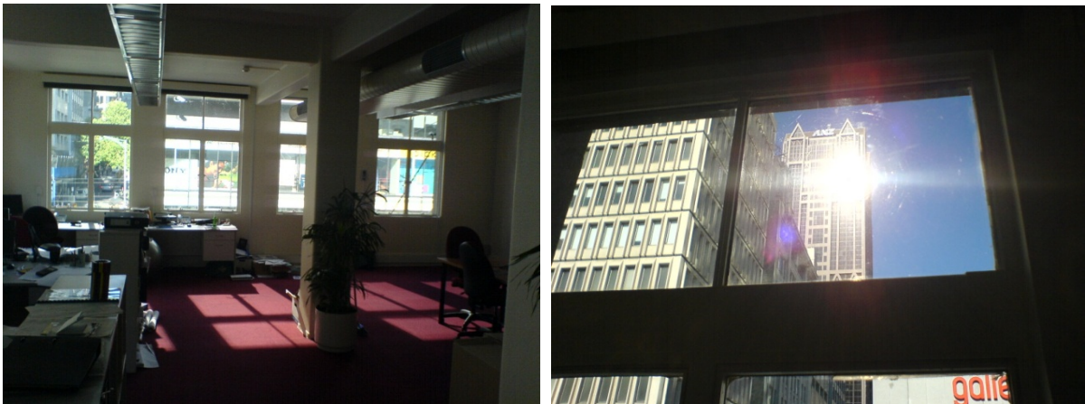
Fig H.13 Glare through west-facing windows at 8 am – Melbourne office on 23 October 2006 (photos: author)
